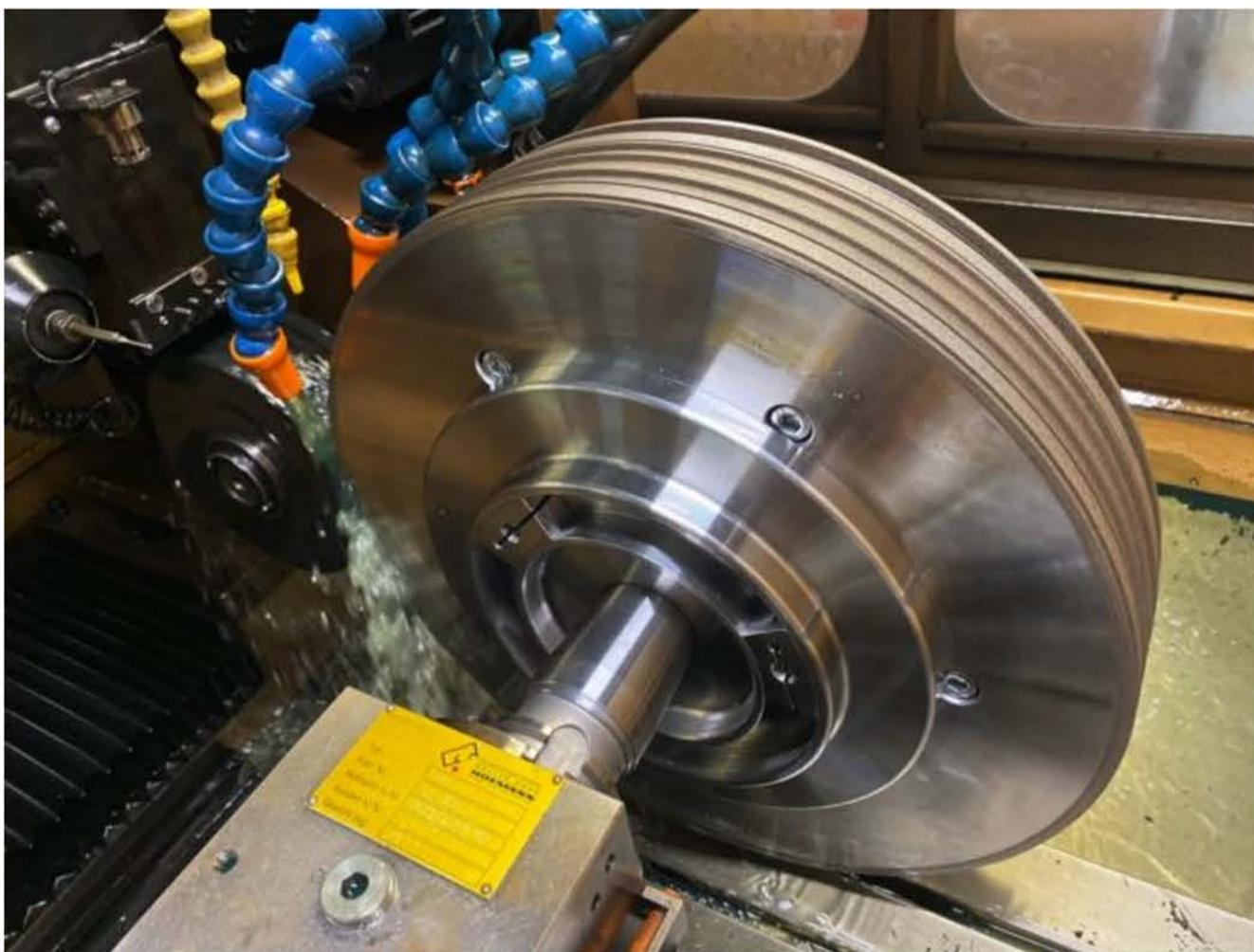
*Deep grinding with »contour-profiled«, metal-bond diamond and CBN profile grinding wheels, showing a 400 mm-dia. CBN grinding wheel on a mini »contour-profiled« spark grinding machine EDG-plus.*
