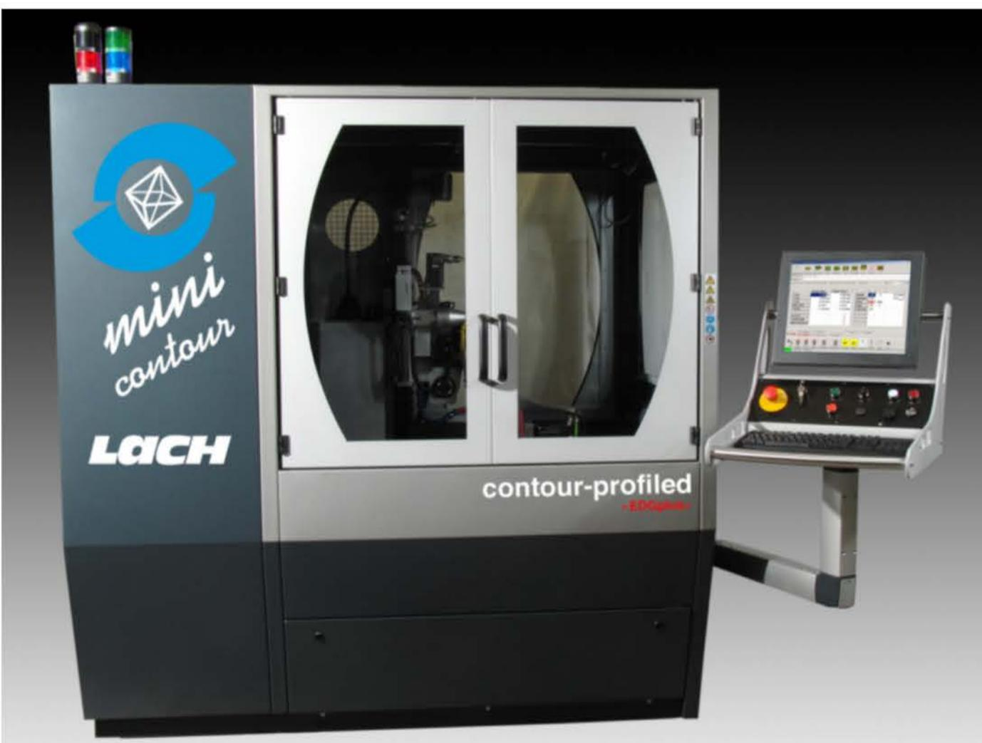
*The »contour-profiled« spark grinding machine EDG-plus by Lach Diamond.*
