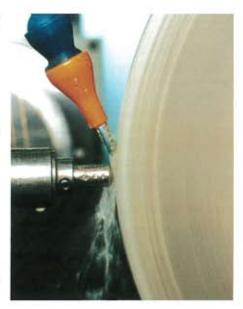
were used for the machining of wood and plastics. Moreover, the idea was born to use these new PCD milling cutters (introduced as "drebojet") for the mill dressing of grinding wheels, a world first. LACH DIAMANT then filed the appropriate patent applications and claims.
